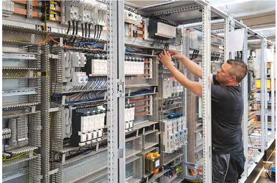
*The often multiple-field switch cabinets are constructed in-house at BSG, wired, tested and shipped worldwide.*
