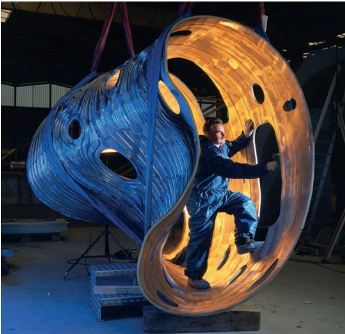
Man-sized tube of the plasma vessel in which the plasma is eventually formed.
