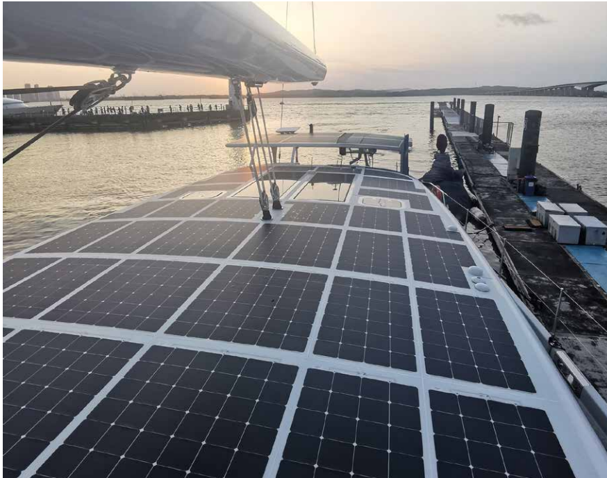
Optimized solar modules make use of even the smallest available surfaces on board to maximize energy generation.
