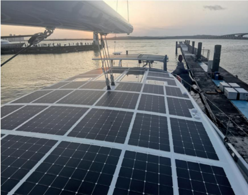
*Optimised solar modules make use of even the smallest available surfaces on board to maximise energy generation.*
