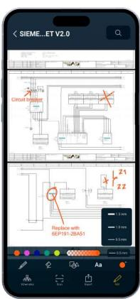
With the new Redlining feature in WSCAD's Cabinet AR App, service technicians and maintainers can document changes directly on-site within the electrical documentation - ensuring up-to-date, understandable records available to everyone at any time.
