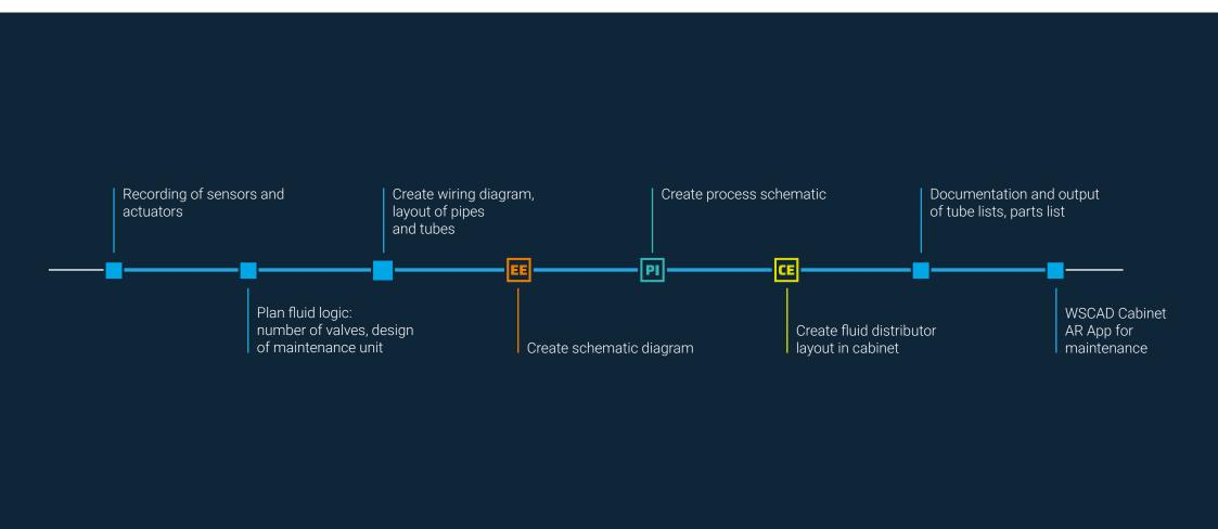
The design and documentation of pneumatic and hydraulic machines and plants are carried out with the help of the Fluid Engineering discipline (FE). This includes all the benefits of WSCAD engineering software, supplemented by special fluid functions such as the logical connections between components or the automatic naming of tubes, for example.
