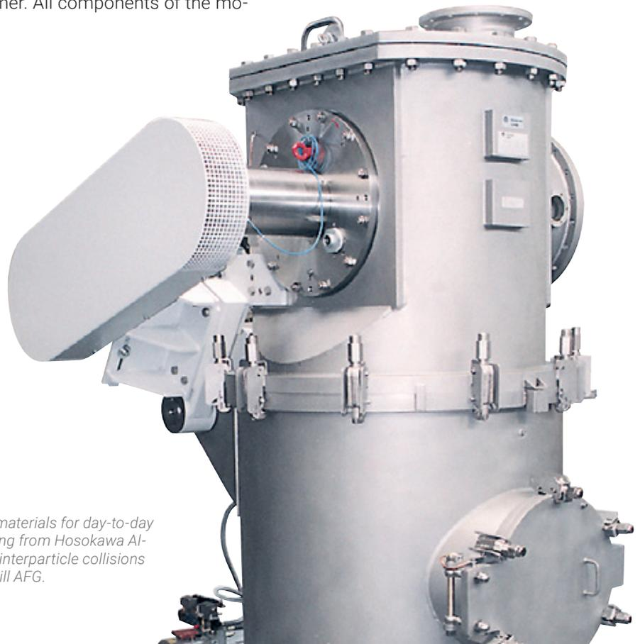
*Powders, granules or bulk solids – many of the starting materials for day-to-day life products are crushed by high-quality machines coming from Hosokawa Alpine based in Augsburg. For example jet milling through interparticle collisions within the gas jets with the Fluidized Bed Opposed Jet Mill AFG.*
